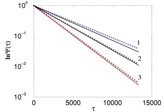
FIG. 3. ACF envelopes (*solid lines*) obtained experimentally for different rms values of the external noise intensity: 1— $D=0$ , 2— $D=0.0005$  mV, and 3— $D=0.001$  mV, and their exponential approximations (*dashed lines*) with the decrement of decay  $B_{\text{eff}}=0.00024$ ,  $B_{\text{eff}}=0.00033$ , and  $B_{\text{eff}}=0.000439$ , respectively. The other parameters for numeric calculations are  $N=100$ ,  $n=262144$ , and  $p=1/2n$ .
