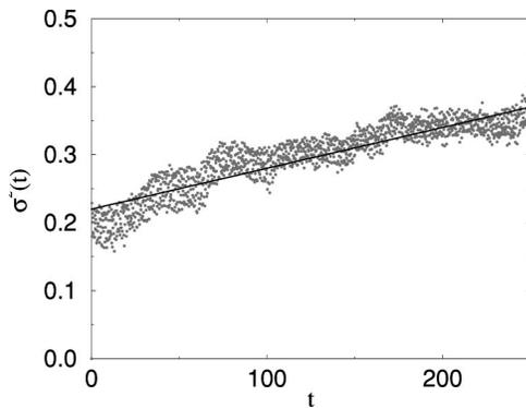
FIG. 2. Temporal dependence of the phase variance in the presence of noise with a root-mean-square value of the noise intensity  $D=0.001$  mV and its linear approximation by the least-square method (time  $t$  is a dimensionless variable and equals the number of periods of oscillations).
