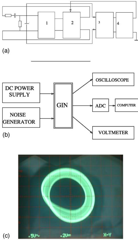
FIG. 1. Schemes of a generator with inertial nonlinearity (a) (1,2—amplifiers, 3—linear amplifier, 4—inertial converter) and of an experimental unit (b), and a picture of the spiral attractor on the oscilloscope screen (c).
