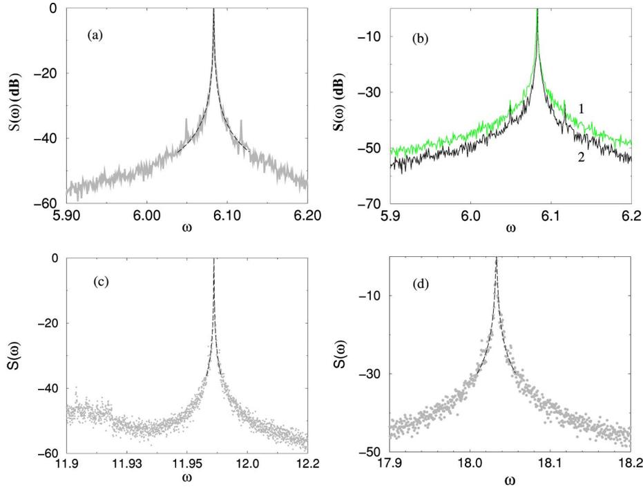
FIG. 4. (a) Experimental power spectrum of the  $x(t)$  oscillations in the GIN and its theoretical approximation by Eq. (5) with  $B_{\text{eff}}=0.00033$  in the presence of noise with  $D=0.0005$ ; (b) power spectra for  $D=0.001$  (curve 1) and  $D=0$  (curve 2); power spectra at the harmonics  $2\omega_0$  with  $2.4B_{\text{eff}}$  (c) and  $3\omega_0$  with  $4B_{\text{eff}}$  (d), where  $B_{\text{eff}}$  is the experimentally found phase diffusion coefficient (see Fig. 2).
