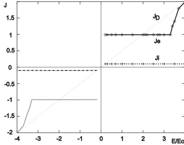
**Fig. 7** Electron-ion stationary currents corresponding to the case of dissipative solitons stabilized by negative friction  $\mu = 0.25$ , as functions of the field strength. The dashed straight line gives for comparison the linear Ohm-Drude current.
