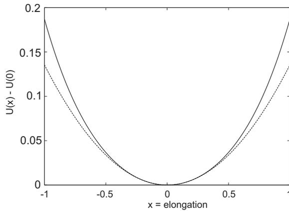
**Fig. 2** The effective potential acting on an ion oscillating between two fixed neighbours at distance  $2\sigma$  in comparison with the harmonic approximation. The minimum corresponds to the equilibrium configuration of the central ion.
